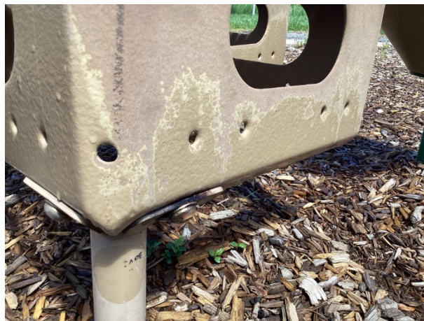
Finish deterioration and minor fastener rust
